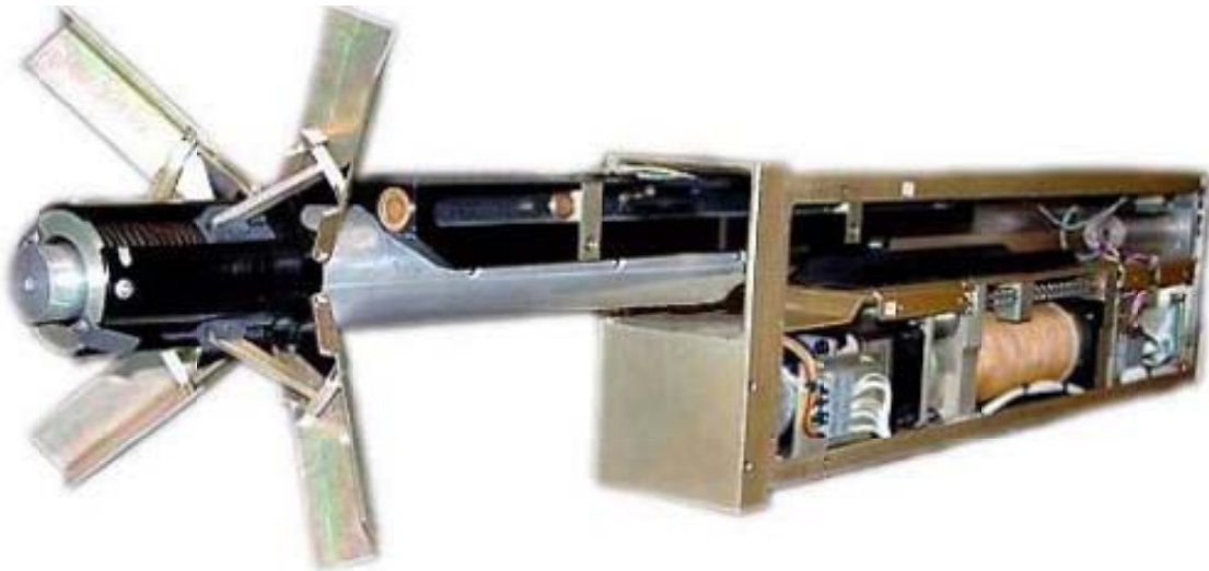
Figure 3-12: Typical Fibre Optic Towed RF Decoy – AN/ALE-55 – (BAE SYSTEMS Photo).
