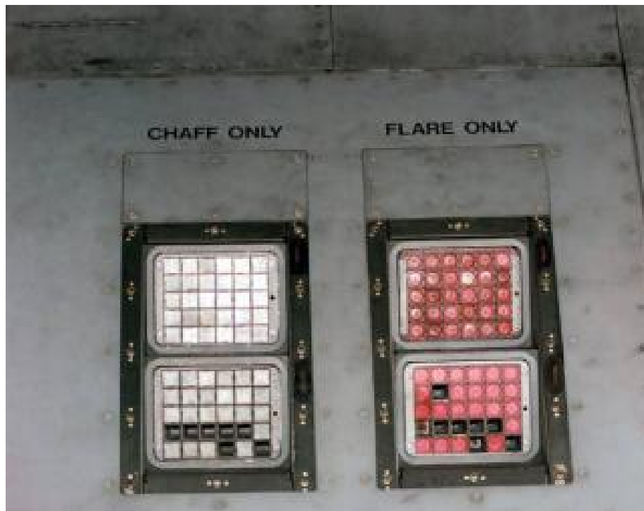
Figure 3-22: CMDS with Magazines Installed on a C-130 – (U.S. DoD Photo).
