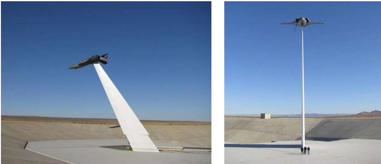
Figure 3-26: F-35 Model Undergoing RCS Measurements – (Lockheed Martin Photos).
